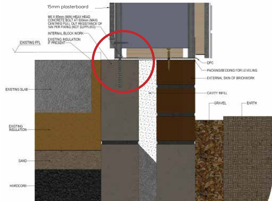
250mm Cavity Wall Base Detail (standard)
