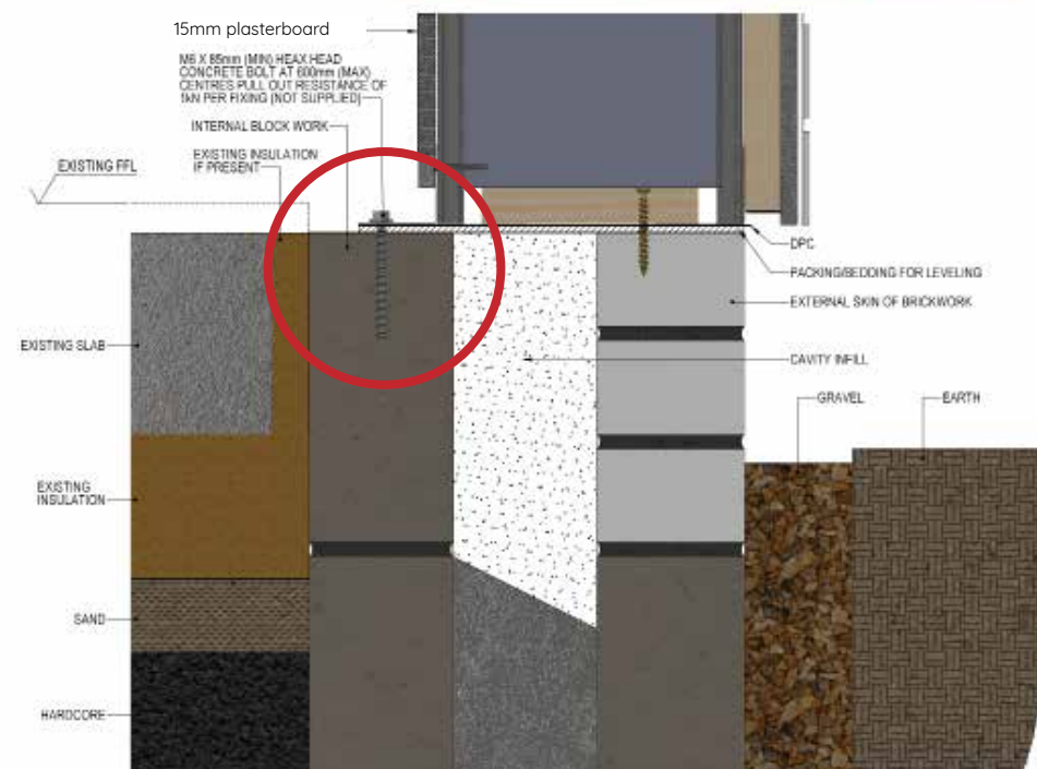
300mm Cavity Wall Base Detail (extended)
